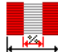
When satin sewing is performed, the ratio of the width of the bobbin thread to the swing width when viewed from the back side.
