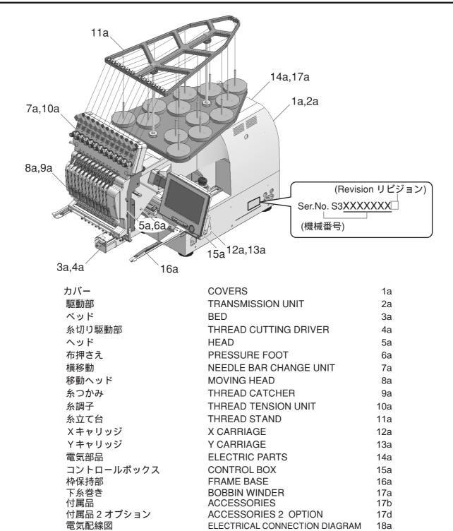
When you place parts orders, please state machine model (example : HCS3-1201-30), machine number and if machine is with option or not.
